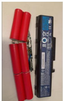
Li-ion battery degraded in real conditions
